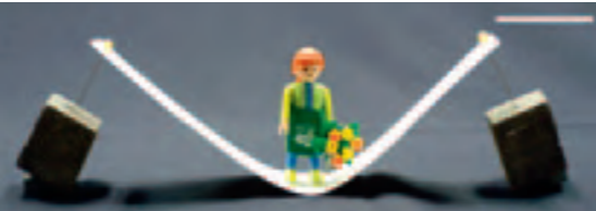
Form of cross section: flat profile Distortion: strong bend – very low load bearing capacity
