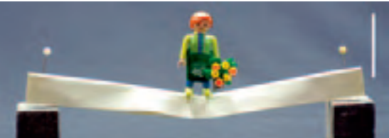
Form of cross section: flat profile; vertically positioned Distortion: twisting along the lateral axis – low load bearing capacity
